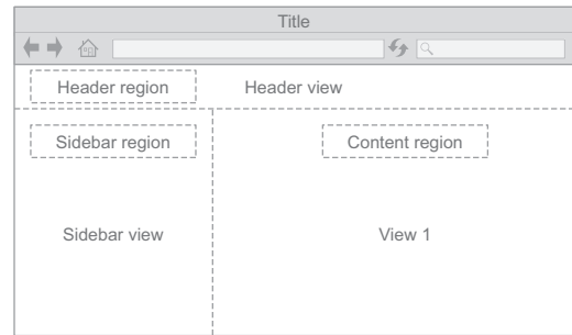
Figure 1.4 Subsections of the shell are called regions. A region’s content is provided by a view.
