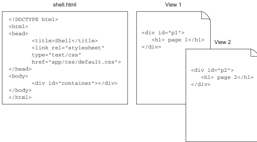
Figure 1.6 In an SPA design, one complete HTML file contains placeholders for the HTML fragments stored in view files.
