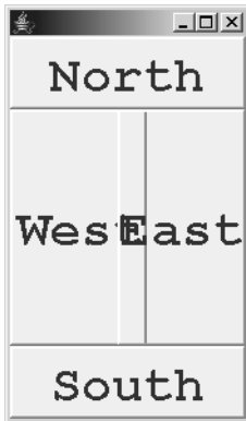
Figure 5-12. BorderLayout horizontally resizes the EAST and WEST components as the container height changes.
