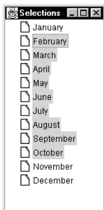
Figure 7-28. The anchor selection (February in this case) is the first node in a range selected, and the lead selection (October) is the node at the opposite end of the selection range.
