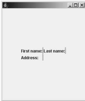
Figure 5-34. GridBagLayout uses preferred sizes if enough space is available but reverts to the minimum size if necessary.
