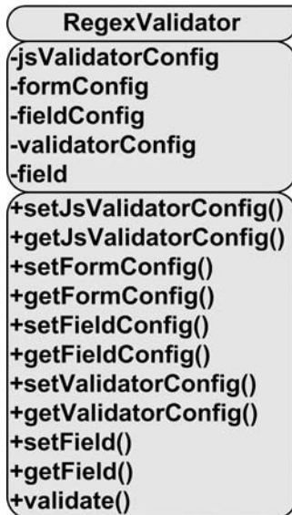
Figure 8-17. UML diagram of the RegexValidator class
