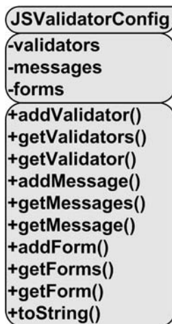
Figure 8-8. UML diagram of the JSValidatorConfig class
