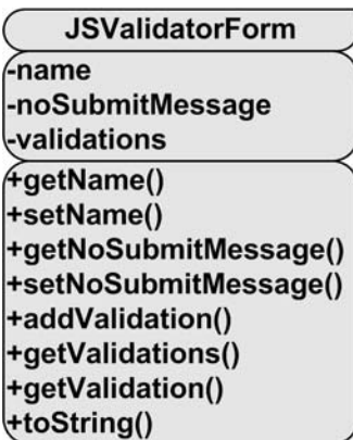
Figure 8-11. UML diagram of the JSValidatorForm class
