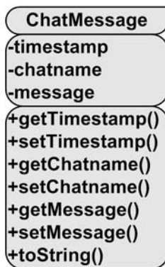
Figure 12-9. UML diagram of the ChatMessage class
