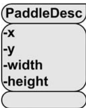
Figure 11-20. UML diagram of the PaddleDesc class
