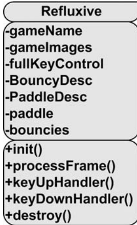
Figure 11-18. UML diagram of the Refluxive class
