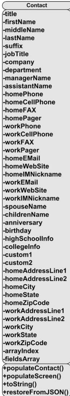
Figure 6-11. UML diagram of the Contact class
