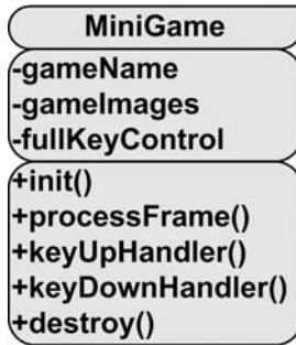
Figure 11-10. UML diagram of the MiniGame class
