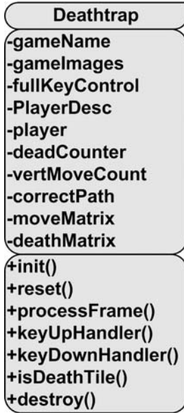
Figure 11-16. UML diagram of the Deathtrap class
