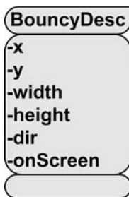
Figure 11-19. UML diagram of the BouncyDesc class
