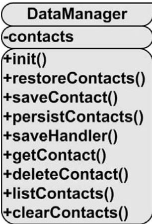
Figure 6-13. UML diagram of the DataManager class
