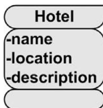
Figure 5-5. UML diagram of the Hotel class
