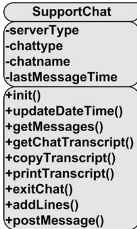
Figure 12-6. UML diagram for the SupportChat class
