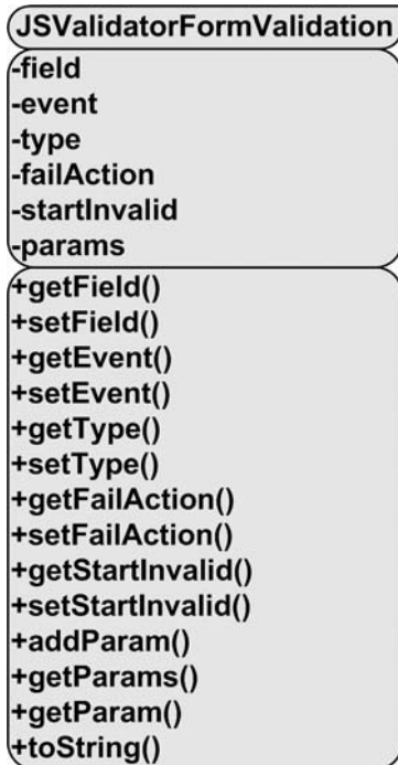
Figure 8-12. UML diagram of the JSValidatorFormValidation class
