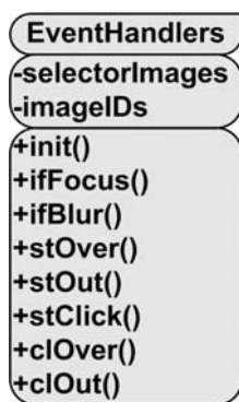
Figure 6-10. UML diagram of the EventHandlers class
