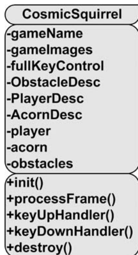
Figure 11-12. UML diagram of the CosmicSquirrel class
