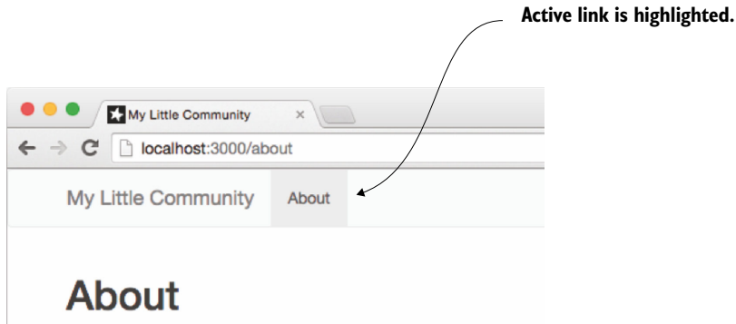
Figure 8.13 An active navigation item has a CSS class active and a highlighted UI.
