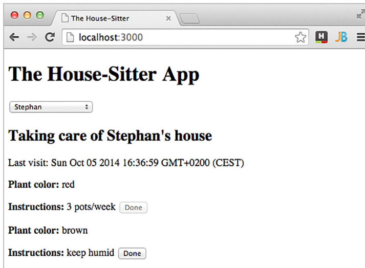
Figure 4.7 The timestamp gets updated onscreen and inside the database by each click on a Done button.
