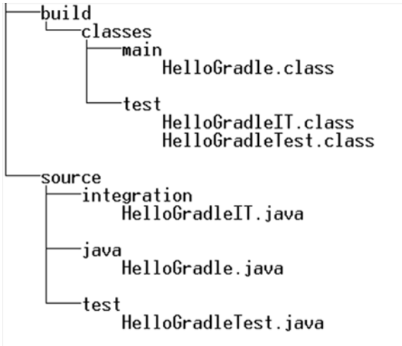
Figure 5-3. Gradle project nondefault layout
