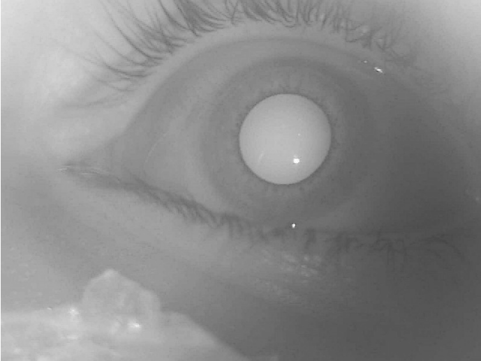
Figure 12.2: Example of eye image showing the bright pupil and the corneal reflection or “glint” [Joshi and Barreto 07].
