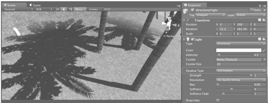
Figure 21.17: Angle modification of directional light.
