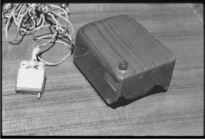
Figure 1.3: Engelbart’s mouse. (With permission from SRI.)
