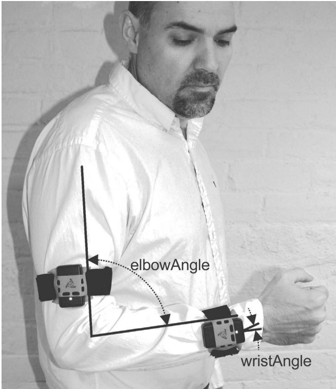
Figure 20.7: Sensor placement for joint angle measurement.
