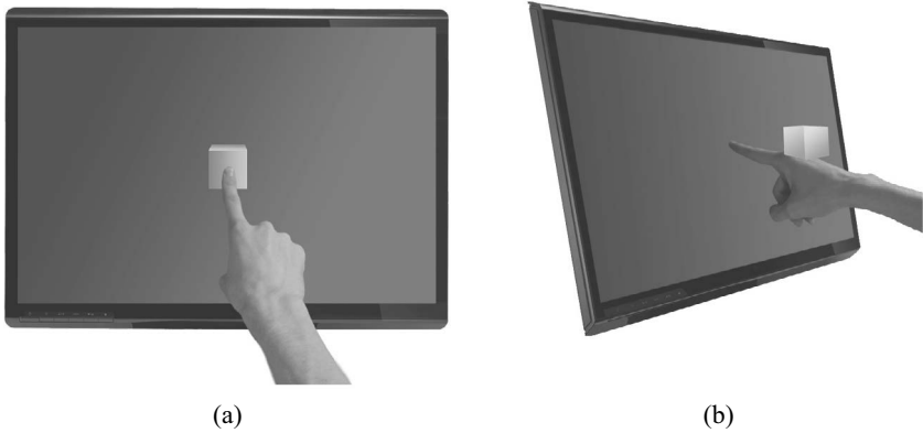
Figure 9.2: Illustration of the occlusion problem; while the occlusion cues (a) indicate that the user’s finger is in front of an object, binocular disparity cues (b) are suggesting that the user’s finger is behind the object.
