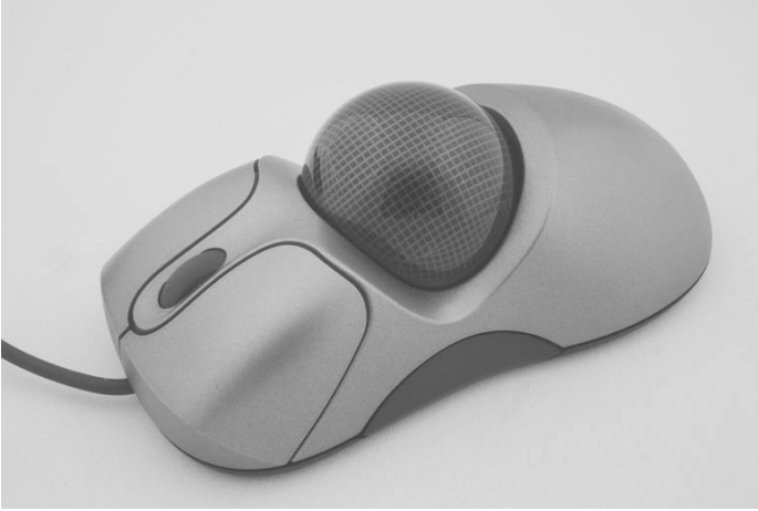
Figure 2.7: Dimentor - Inspector 6DOF trackball mouse, circa 2008 [Buxton 14] . (With permission from Bill Buxton).
