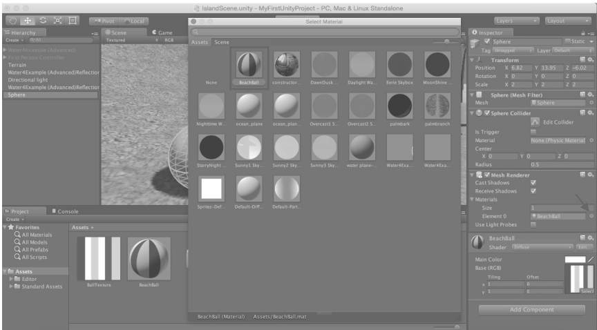
Figure 21.23: Assign the texture image to material.
