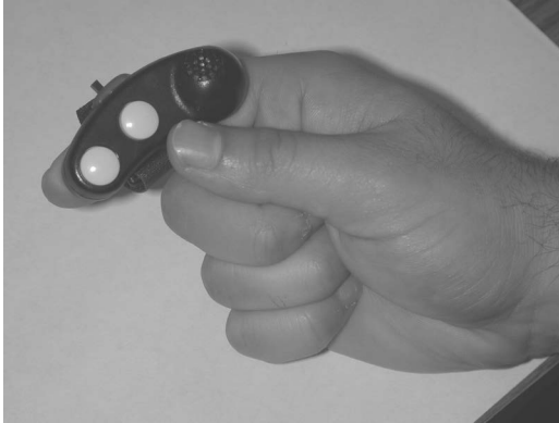
Figure 2.21: The Ring Mouse. Courtesy of Joseph J. LaViola, Jr.
