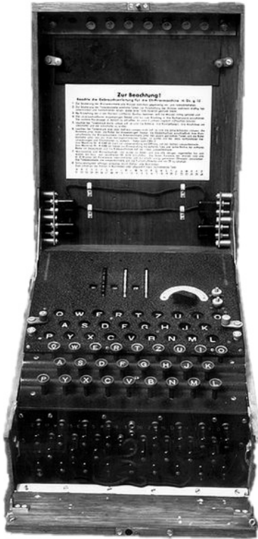
Figure 1-10. German Enigma machine
