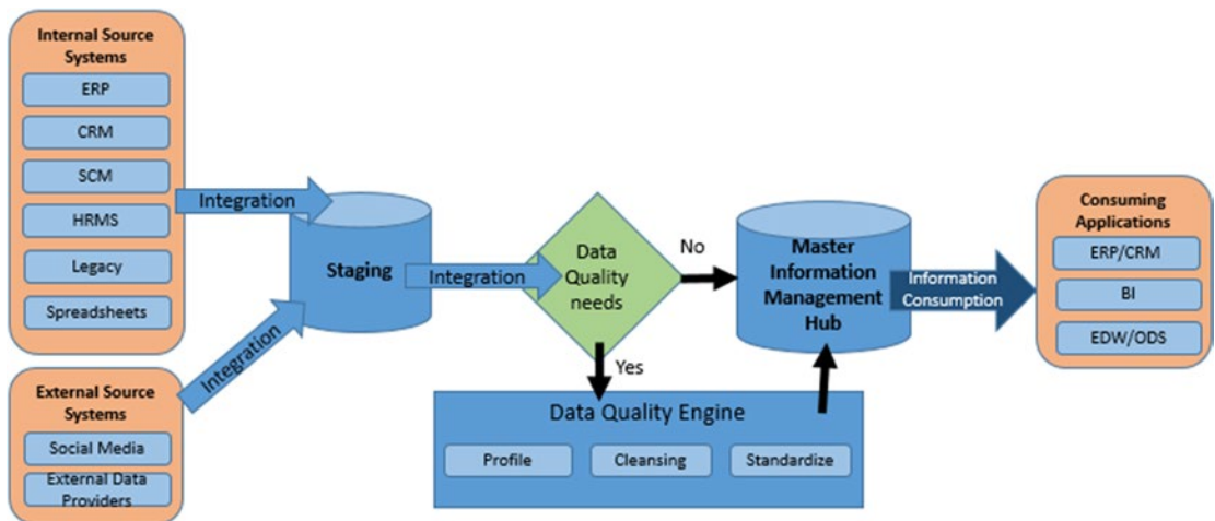
Figure 7-6. Solution architecture of master information management
