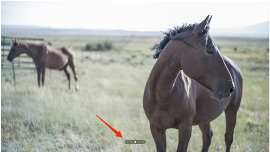
Figure 4-1. An example of a Page View Controller and its associated Page Control
