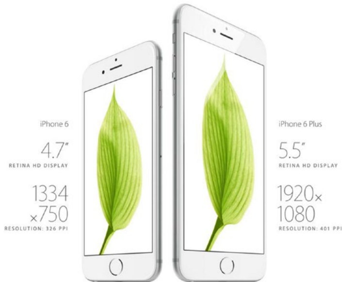
Figure 5-6. The screen resolutions and display sizes of the iPhone 6 and iPhone 6 Plus
