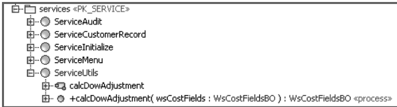
Figure 9.50. Tree structure for “ServiceUtils” and “calcDowAdjustment” as contained element (activity diagram and associated operation)
