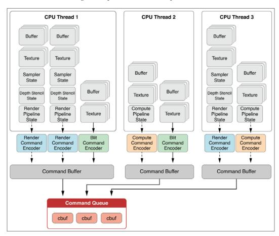
In the previous figure, we can see three threads are submitting work to the command queue in parallel, and each thread has its own command buffer.
