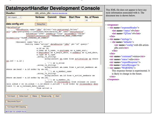
The screen is divided into two panes: on the left is the DIH control form and on the right is the command output as raw XML.
