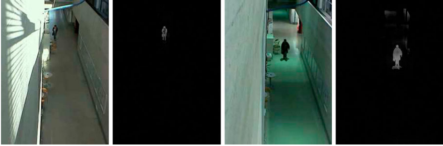
Fig. 13.9 Different illumination conditions with the corresponding background subtracted images. Even in case of totally different illumination conditions and differently appearing objects the background subtracted image gives a similar representation of the object
