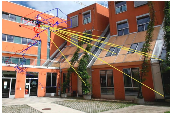
Fig. 7.1 We present an approach to visual localization which exploits prior knowledge in form of pictures taken at ground-level to enhance the accuracy and reliability of position and attitude estimation. Our algorithm ( red trajectory ) is neither prone to drift nor bias and therefore outperforms pure SLAM approaches ( blue trajectory ). ©2011 IEEE. Reprinted, with permission, from [67]
