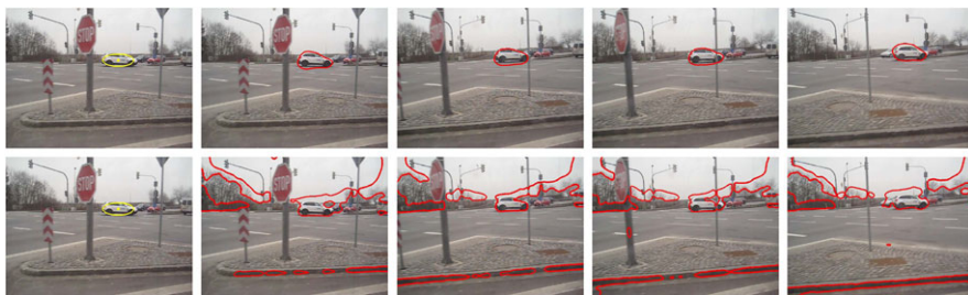
Fig. 8.13 Moment constraints for object tracking. The user initializes the tracking in form of an ellipse in the first frame (left), from which histograms and constraint parameters are derived. The first row shows results with moment constraints, where a deviation of the centroid is allowed from each frame to the next one to account for the object's motion. The second row shows results of histogram based tracking without constraints. This comparison shows that moment constraints can realize acceptable real-world object tracking with no previous learning of shapes
