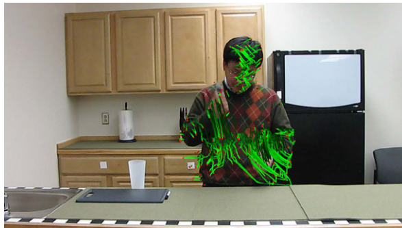
Fig. 4.2 Messing et al.’s sparse features found on another sample frame from URADL’s Answer Phone activity. Red dots denote feature candidates. Green trails denote trajectory histories
