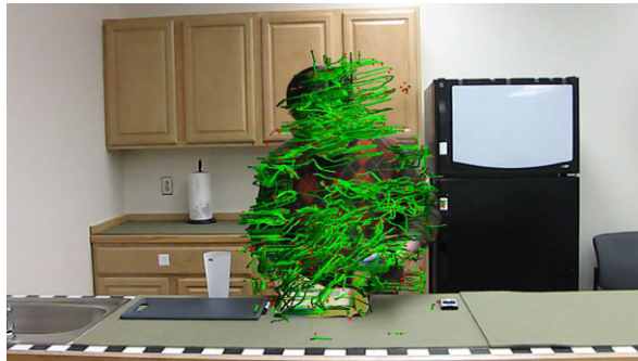
Fig. 4.4 Messing et al.’s sparse features found on another sample frame from URADL’s Lookup in Phonebook activity. Red dots denote feature candidates. Green trails denote trajectory histories
