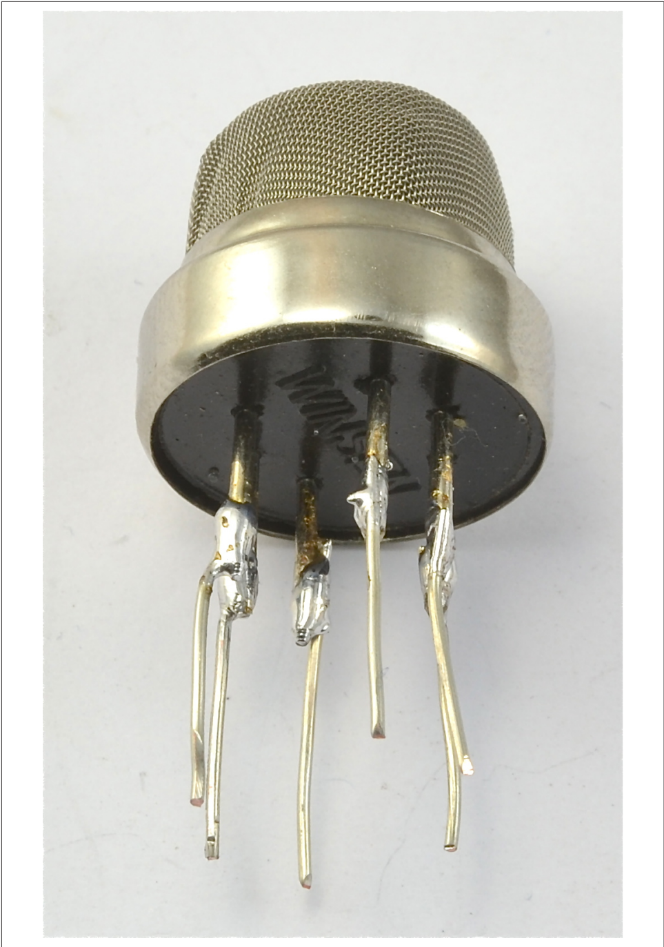
Figure 13-7. Soldering leads onto the gas sensor
