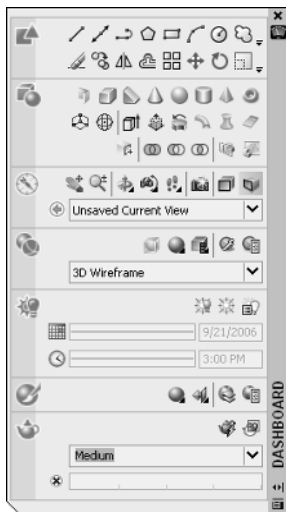
Figure 2-2: Dashboard allows for quick access to a variety of different 3D-related tools.
