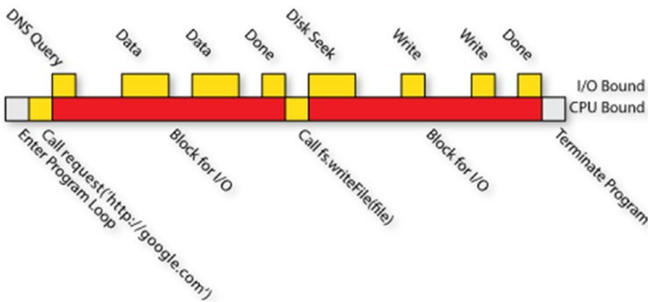
Figure 21-1. Timeline of a synchronous program
