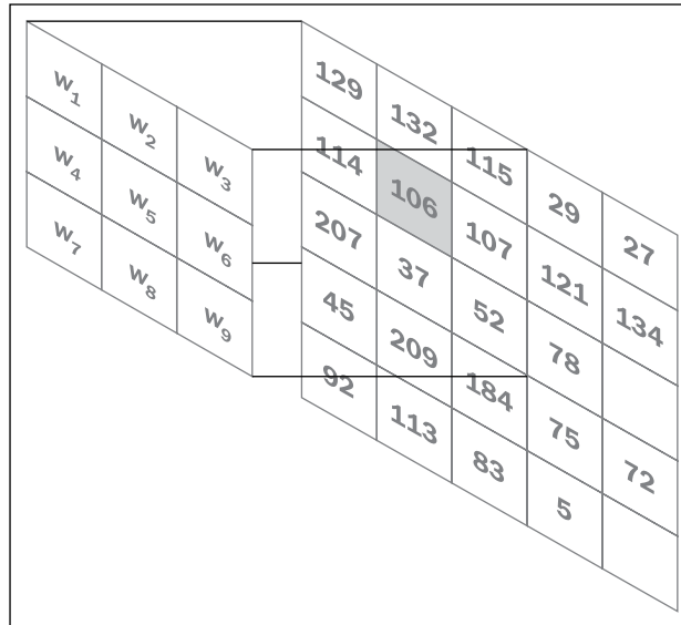
Original image to be processed (right) and convolution mask (left) that contains the weights to be applied to every surrounding pixel.
