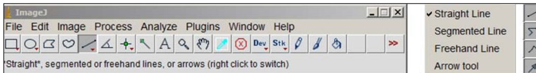
The ImageJ main window with a straight line tool selected (left) and available options for this tools with their corresponding toolbar icons (right).
