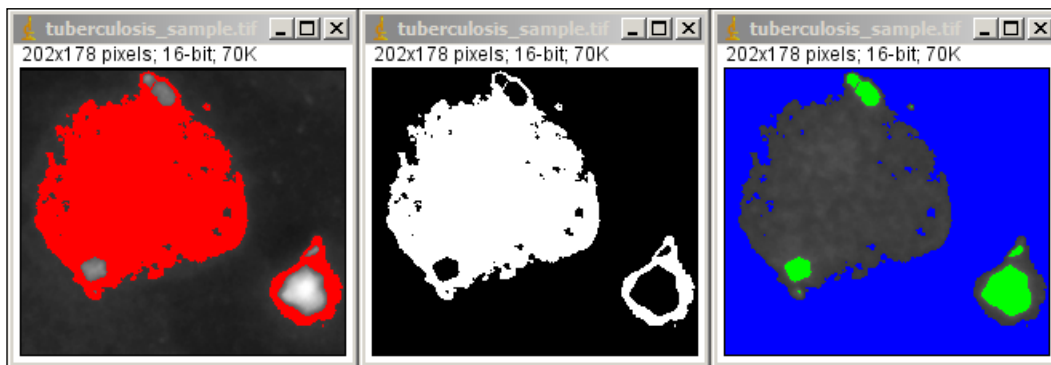
Different visualization modes during the thresholding process: Red (left), B&W (center), and Over/Under (right).
