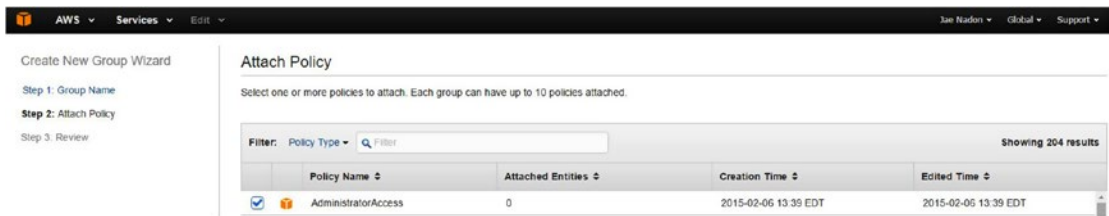
Figure 2-6. The AWS IAM Create New Group Wizard showing the Attach Policy step with “AdministrativeAccess” selected
