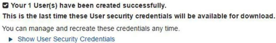
Figure 2-7. The AWS IAM Create User Wizard after the Create button has been clicked. At this point, you can download or view the user security credentials. These credentials are needed for tool or integration access such as the AWS Command Line Interface.
