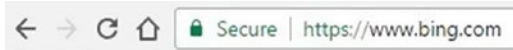
Figure 18-2. A browser client with a secure connection to www.bing.com over the HTTPS protocol
