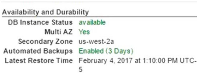
Figure 16-7. The AWS RDS database instance detail configuration for the Availability and Durability section shows that automated backups are enabled and set to three days of backups
