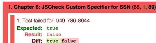
**Figure 6.9** A failure detected as a result of an invalid property check with QUnit. When you randomize the input to include invalid inputs, the JSCheck algorithm has enough entropy that 89 of 90 tests fail.
