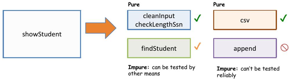
**Figure 6.6** Identifying the testable areas of the `showStudent` program. The components that perform IO are impure and can't be tested reliably because they contain side effects. Other than having impure parts, the scope of the entire program remains highly testable.
