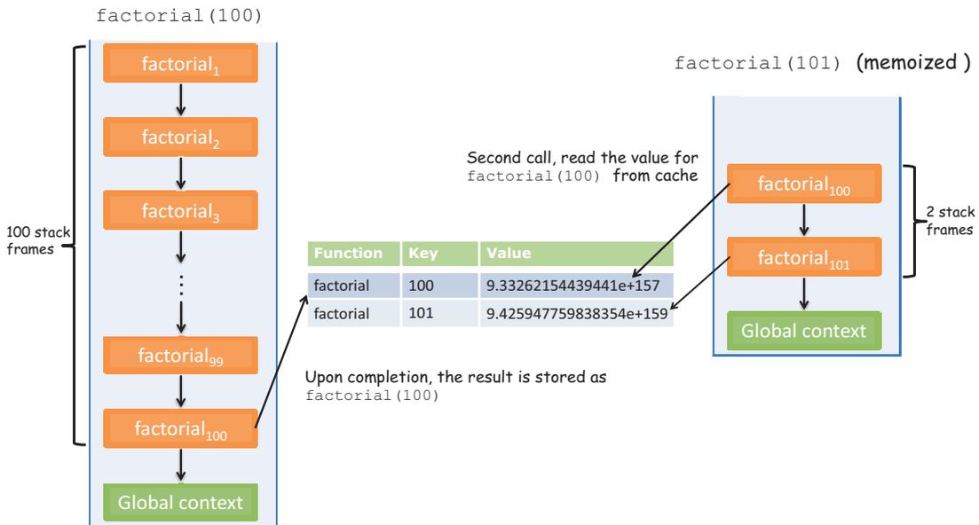
**Figure 7.8** Running the memoized `factorial(100)` the first time creates 100 stack frames because it needs to compute  $100!$  by multiplying every single number. On the second call to `factorial` with 101, via memoization it’s able to reuse the result of `factorial(100)` and create only 2 stack frames.
