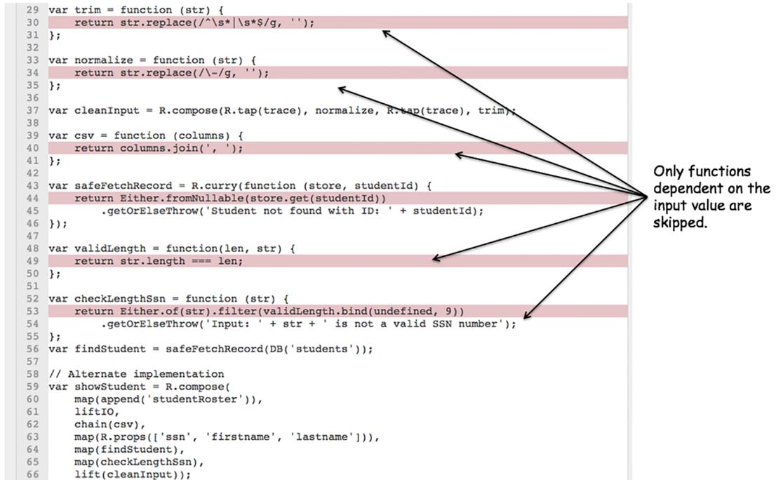
**Figure 6.13** The functional version of `showStudent` skips lines related only to manipulating the data that would have originated from an otherwise valid input.
