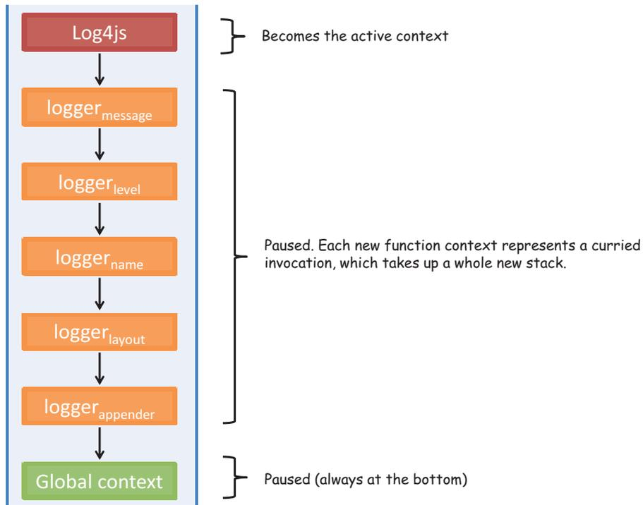
**Figure 7.4** With currying, each parameter of the curried function is internally transformed to a nested call. This flexibility of being able to supply parameters sequentially has the downside of occupying additional stack frames.
