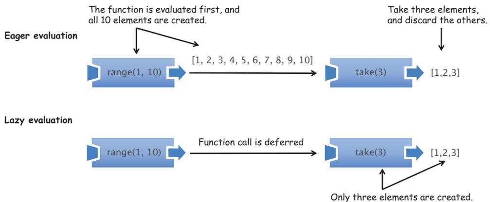
**Figure 7.6** The composition of the function `range` (returns a list of numbers from beginning to end) with `take` (reads the first  $n$  elements). In eager evaluation, the `range` function executes completely, feeding its result to `take`. With lazy evaluation, the result of `range` never executes until the dependent operation, `take`, is called.
