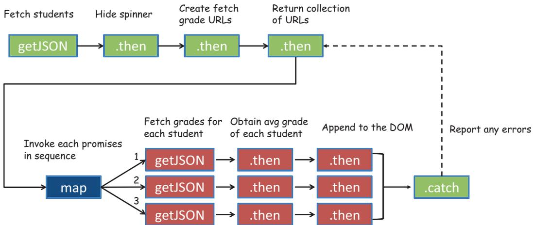
**Figure 8.7** The flow of behavior through the chained use of promises. Each thenable block contains a function that transforms the data passed through it. Although this program is bug-free and has all the desired functional qualities, it's inefficient because it uses a waterfall sequence of `getJSON` requests to fetch each student's grades.
