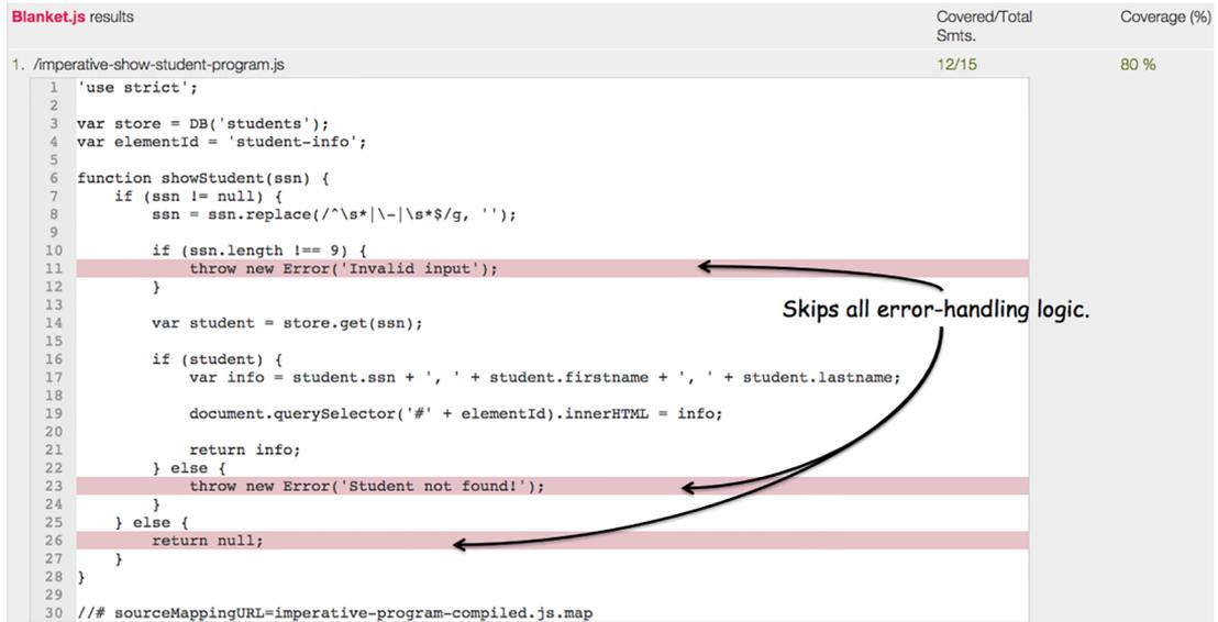
**Figure 6.10** QUnit/Blanket output running the imperative `showStudent` with valid input. The highlighted lines represent statements that never ran. Because 12 of 15 lines ran, this registers only 80% of total coverage information on this function.
