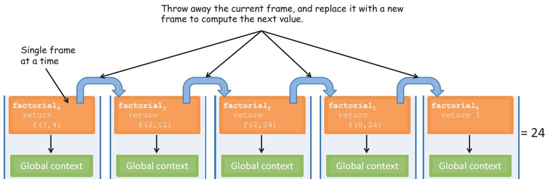
**Figure 7.9** A detailed view of tail-recursive `factorial(4)` evaluation. As you can see, the function uses a single frame. TCO is in charge of throwing the current function frame to give way for a new one, as if `factorial` was being evaluated in a loop.
