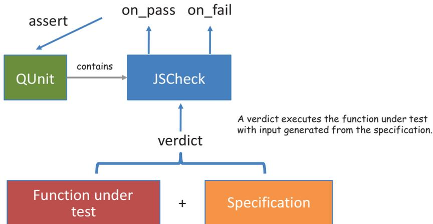
**Figure 6.8** The integration of the main components: JSCheck and QUnit. A QUnit test encapsulates a JSCheck test specification. The specification and the function being tested are supplied to the `verdict` function, which is run through the JSCheck engine to invoke the pass/fail callbacks. These callbacks can be used to trigger QUnit assertions.
