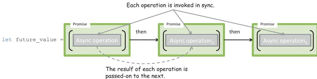
**Figure 8.6** A sequence of chained promises joined via the `then` method. Each `then` clause is executed serially with one promise value after the next as soon as each is fulfilled.
