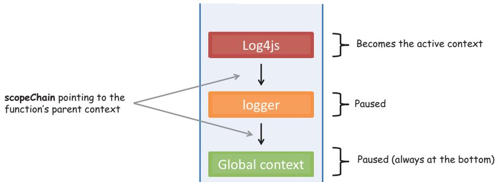
**Figure 7.3** How the function context grows when running nested functions. Because each function produces a new stack frame, the stack grows in proportion to the level of nesting in functions. Both currying and recursion rely on nested function calls.
