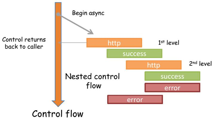
**Figure 8.2** A program’s simple linear control flow breaks down on a remote call and degenerates into a waterfall of nested function calls—a pyramid that grows horizontally like a “Christmas tree of doom.”
