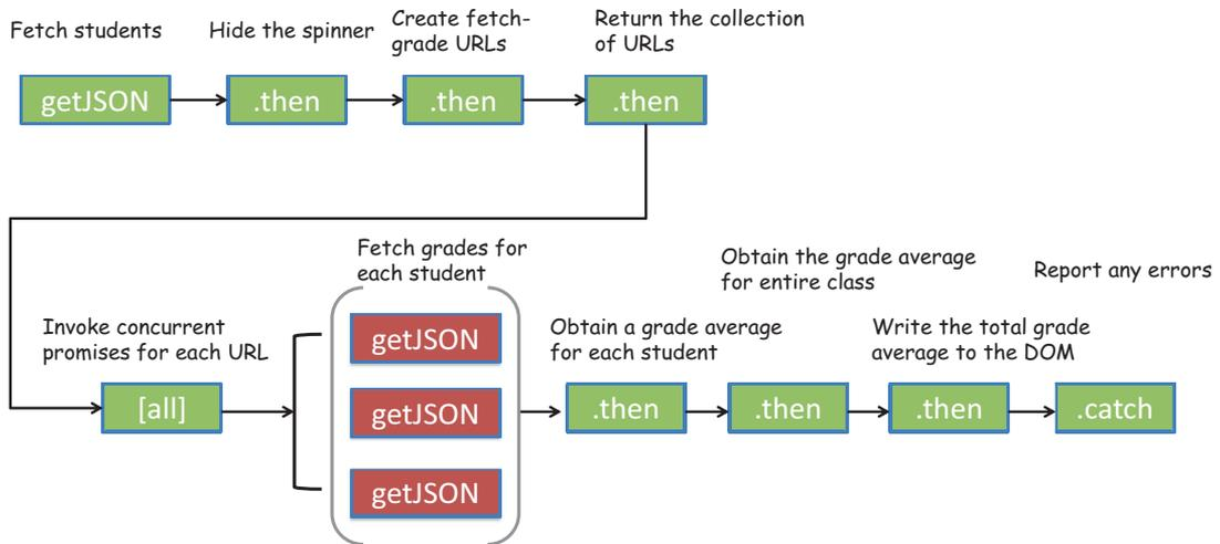
**Figure 8.8** The flow of behavior through the chained use of linear as well as concurrent promises with `Promise.all()`. Each thenable block contains a function that transforms the data passed through it. This program is efficient because it can spawn several parallel connections to fetch all the data at once.
