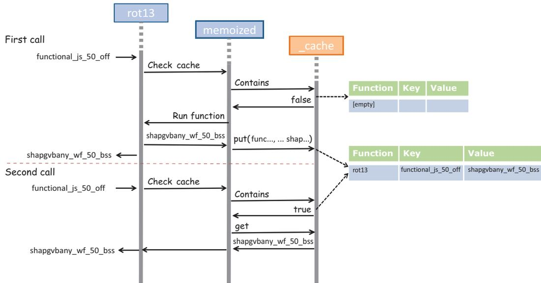
**Figure 7.7** A detailed view of two calls to the `rot13` function with the message “`functional_js_50_off`.” The first time around, with an empty cache, the ROT13 code of the provided discount code is computed. This result is stored in the internal cache with a key generated from this input. The second call results in a cache hit: the value is directly returned without the hash being computed again.
