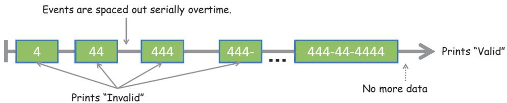
**Figure 8.13** Shows the event values for SSN treated as an observable stream created from subscribing to the change event of the student SSN input field
