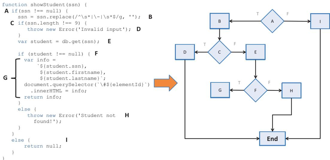
**Figure 6.16** Potential nodes in the imperative version of `showStudent`. These labels have been converted into a flowchart of nodes and edges, which illustrates the number of different linearly independent paths through the code caused by the presence of conditional statements.
