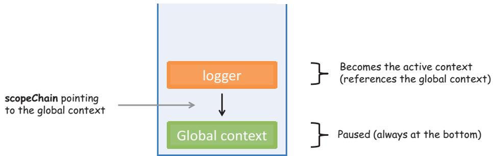
**Figure 7.2** When invoking any function, like `logger` in this case, the single-threaded JavaScript runtime pauses the current global context and activates the context for the new function to run. At this point, a link is created between the global context and the function context, traversable via the `scopeChain`. Once `logger` returns, its execution context is popped off the stack, and the global context resumes.
