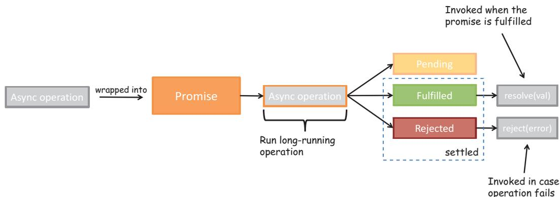
**Figure 8.5** How an async operation is wrapped in a `Promise` and provided with two callbacks: one for `resolve` and another for `reject`. The promise begins with a status of pending and then is either fulfilled or rejected, invoking the function `resolve` or `reject`, respectively, before moving into the settled state.
