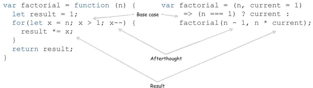
**Figure 7.10** The similarities between a standard loop (left) and its equivalent tail-recursive function. In both code samples, you can easily see the base case, the afterthought or accumulated parameter, and the result.
